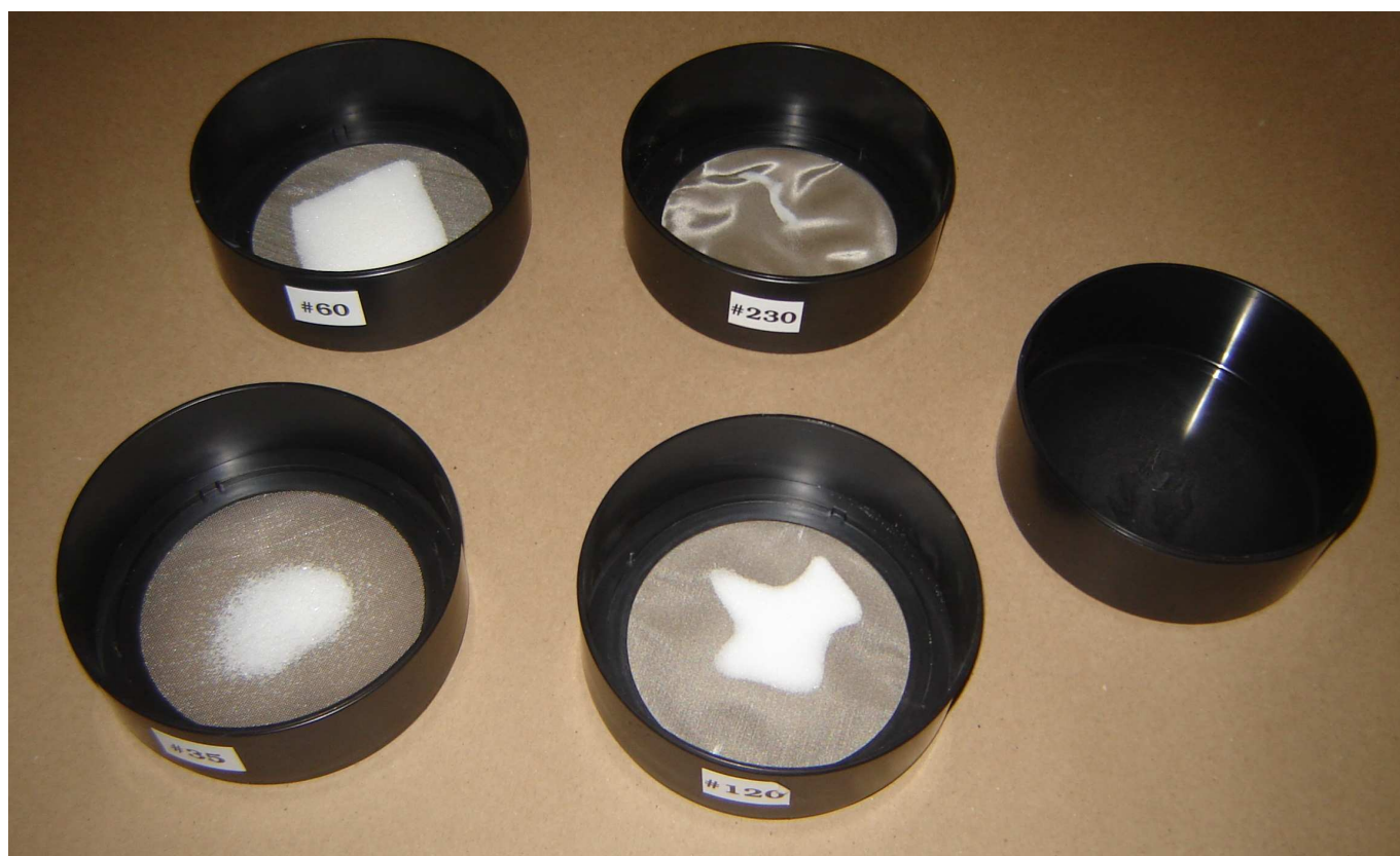
Figure 2 Sieves and pan with sugar retained.
