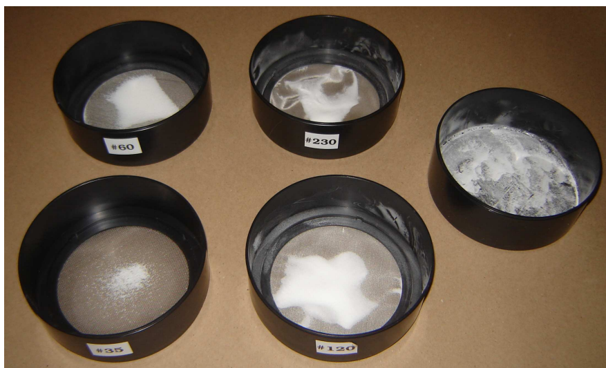
Figure 2 Sieves and pan with \text{KNO}_3 retained.
