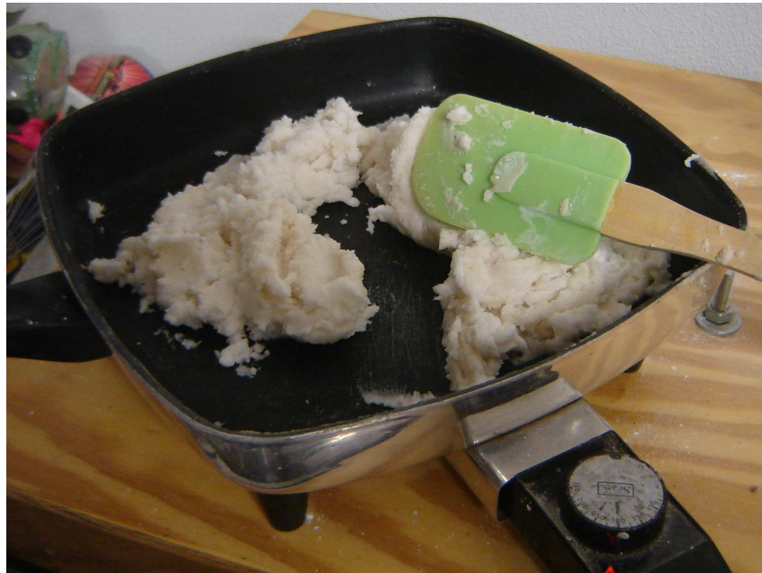
Figure 3 Propellant made of Skylighter \text{KNO}_3 and sorbitol.
