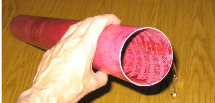
Aft chamber thermal liner fabricated from Deltaflex-100
