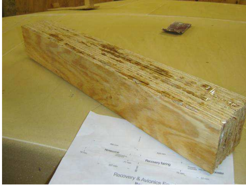
14-ply bonded plywood block for nosecone plug-mould
