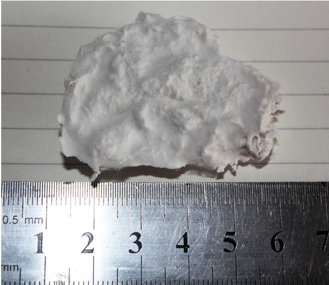
Fig. 7 \text{KNO}_3 - \text{NaNO}_3 -Mannitol propellant reinforced by cotton fibers, after curing
