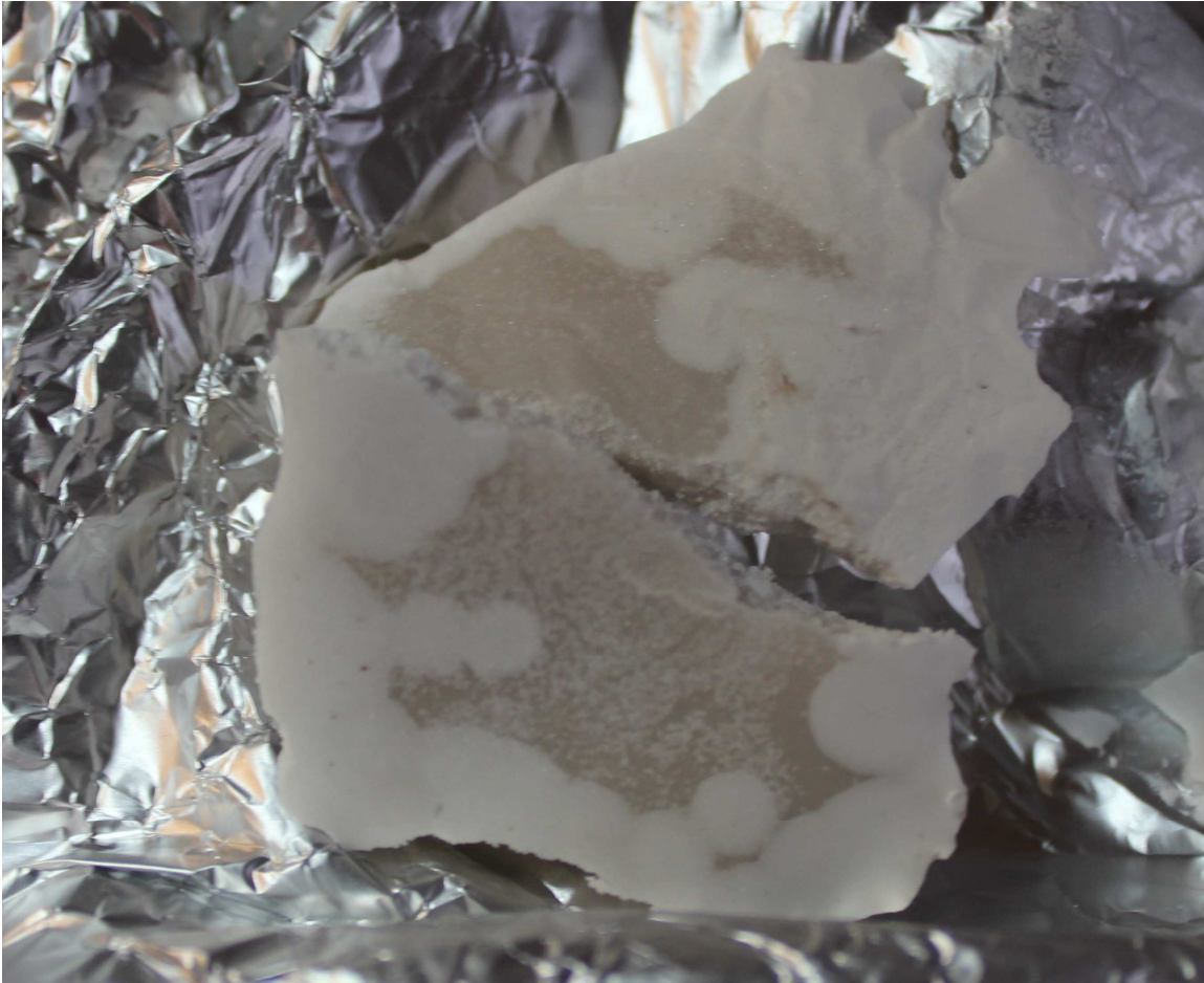
Fig. 3 Chunks of eutectic \text{KNO}_3 - \text{NaNO}_3 -Mannitol propellant starting to cure
