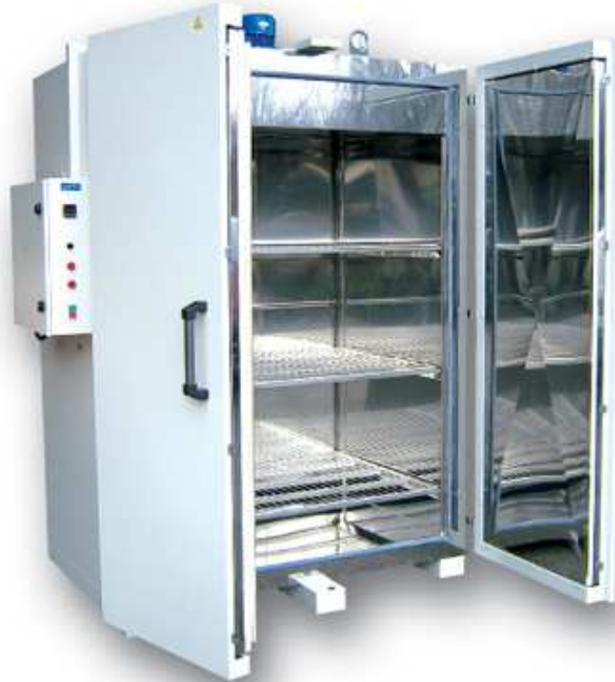
Fig. 4 Example of a suitable industrial oven from france-etuves.com. Temperature spatial variation: less than \pm 1,2^\circ\text{C} at 105^\circ\text{C} and less than \pm 2,5^\circ\text{C} at 200^\circ\text{C} . The oven is available with an internal height of 500mm to 1800mm and max. temperature up to 300^\circ\text{C} [9]
